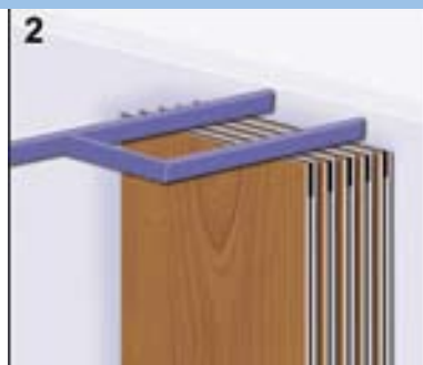
2 Elements with two wheel assemblies, with the second wheel staying on the main track.
