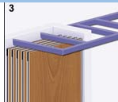
3 Elements with two wheel assemblies, with elements that have been completely moved away from the main track.
